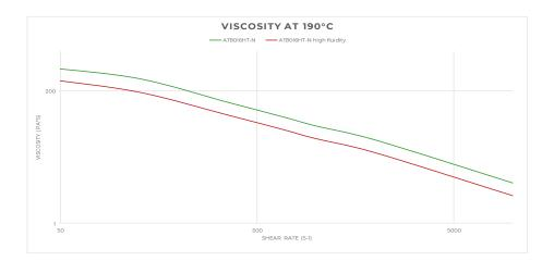
Example for standard high temperature viscosity grade (AT8016HT-N) and improved viscosity grade (AT8016HT-NHi fluidity)
